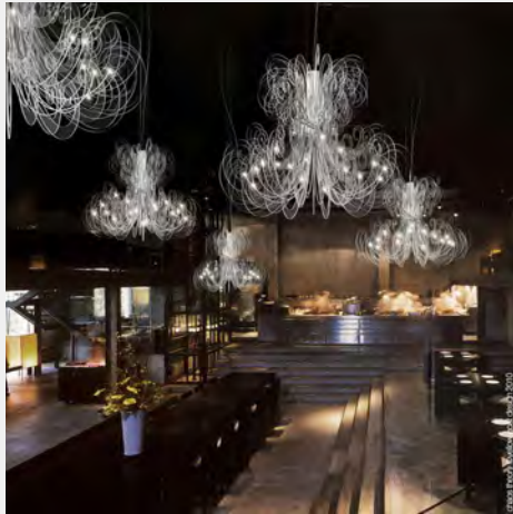
CHAOS THEORY DIMENSION - Ø4'-0" PER ELEMENT MATERIAL - ACRYLIC LIGHTING - LED BI-PIN
