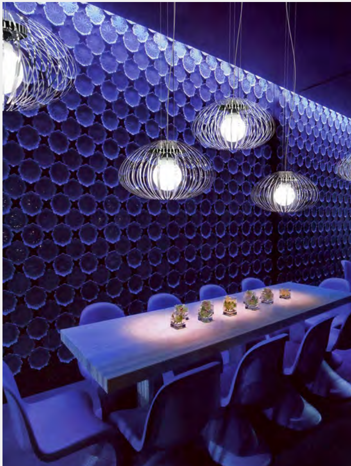
CILLA DIMENSION - Ø1'-8" X 1'-0" H PER ELEMENT MATERIAL - ACRYLIC LIGHTING - LED
