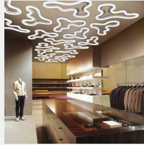
ELL DIMENSION - 3'-3" X 2'-8" H PER ELEMENT MATERIAL - ACRYLIC LIGHTING - LED
